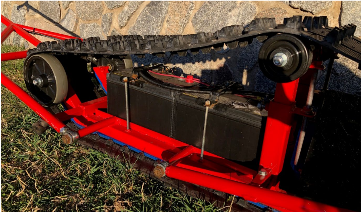
The mule is powered by two car batteries.
